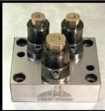
Standard Units Adapted to Existing Special Retainer
